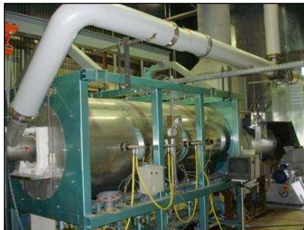
Figure 3. 1 MWth oxy-combustion test rig at Air Liquide's CRCD.
