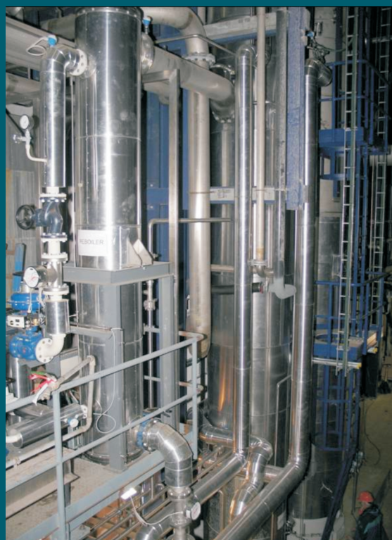
The 1 t/hour CO 2 capture pilot plant using an amine wash process that is installed at the Elsam Esbjerg power plant in the framework of the EC CASTOR project (courtesy of IFP)
