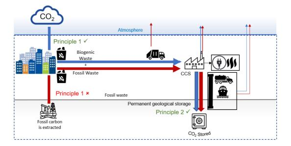
[Figure from report "Europe needs robust accounting for carbon dioxide removals", showing an example of a waste-to-energy plant with CCS. Biogenic (blue) and fossil (red) carbon flows, leakages, heat and power outputs are indicated in the process. For legend, view the ZEP report.]
