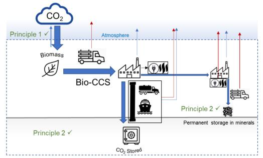
[Figure from report "Europe needs robust accounting for carbon dioxide removals", showing an example of a mineralisation. Biogenic (blue) carbon flows are represented together with and fossil (red) leakages, while heat and power outputs are indicated in the process. For legend, view the ZEP report.]
