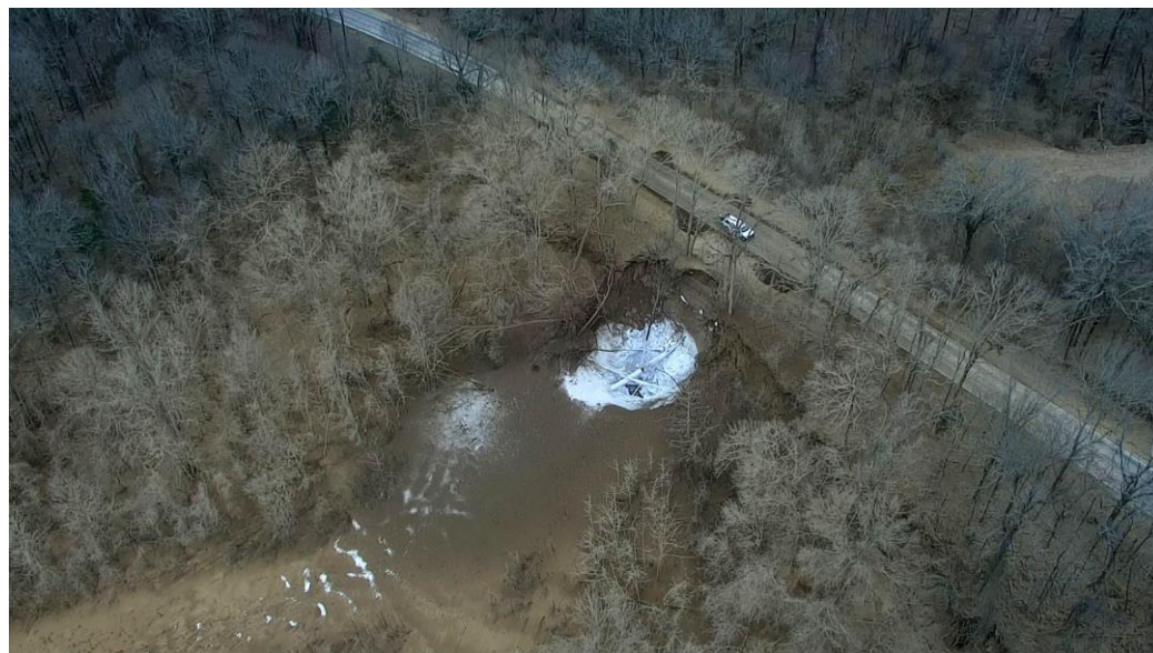
Figure 6: Aerial photograph of a CO 2 leakage from the rupture of a Denbury Resources CO 2 pipeline in Yazoo County Mississippi, USA on 22 February 2020
