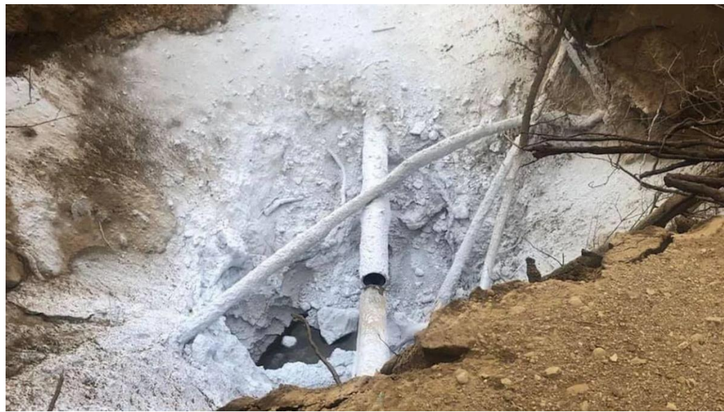
Figure 7: Close up photograph of a CO 2 leakage from the rupture of a Denbury Resources CO 2 pipeline in Yazoo County Mississippi, USA 22 February 2020 showing localised freezing caused by the Joule Thompson effect
