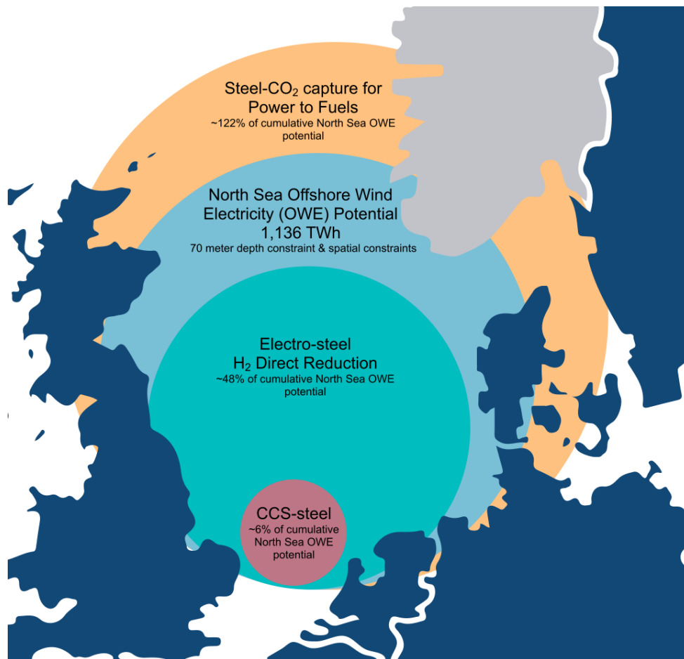
Figure 3 North Sea Offshore Wind Electricity (OWE) potential, 132,000 km 2 with 1,136 TWh (Cameron, et al., 2011). Comparison of electricity requirement for EU low carbon steel manufacture with CCS, electrolysis of hydrogen and direct reduction, CO 2 conversion via power to fuels. Producing new electro-steel in Europe at current production volumes would monopolise almost 50% of the total practical renewable wind electricity potential of the North Sea. Production of power to fuels of EU new steel CO 2 would exceed all North Sea offshore wind generation potential 13
